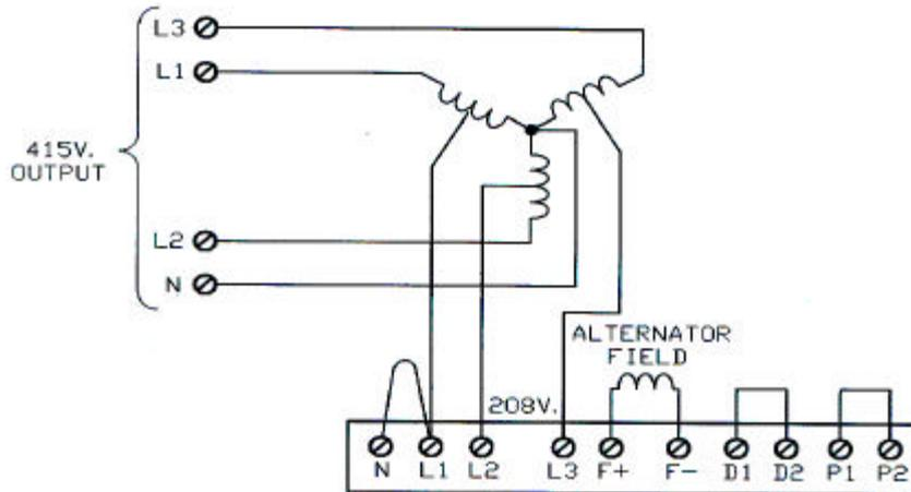
415 Volt Alternator with 3Ø 3 wire centre tap (208V) sensing & supply .
